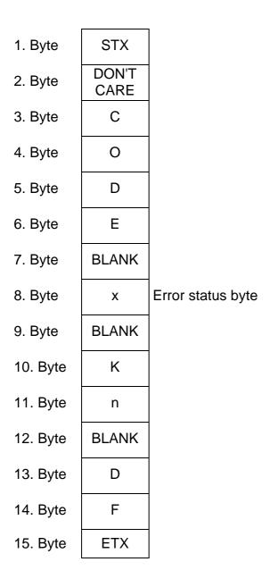
Error status byte: Value is zero: Device without error. Value is not zero: Device with one or more errors.
